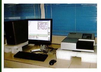
A new automated system to identify bacteria and fungi based on conventional phenotypic tests has been installed at IISR, Calicut. The Biolog System rapidly identifies over 1,900 species of aerobic bacteria, anaerobic bacteria, yeast and filamentous fungi. This easy to use System provides reference laboratory quality identifications without the labour-intensive conventional microbiological assays.
